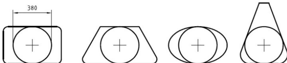
**Figure 1 - Measurements of Minimum Clear Opening**
